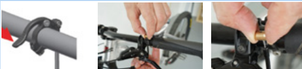
Figure 163: Removing the cartridge
