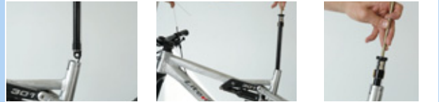
Figure 189: Fastening the cartridge valve lid
