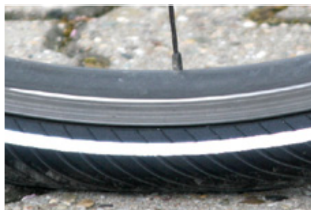
Figure 103: Correct tyre pressure. The tyre is barely deformed under the load of the body weight
