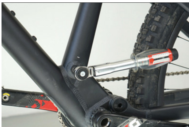
Figure 87: Tightening the seat post axle
