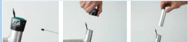
Figure 203: Removing the outer sleeve and slide bushing
