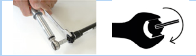
Figure 183: Setting in a clockwise direction
