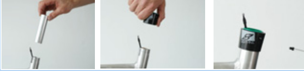
Figure 218: Fitting the slide bushing and outer sleeve
