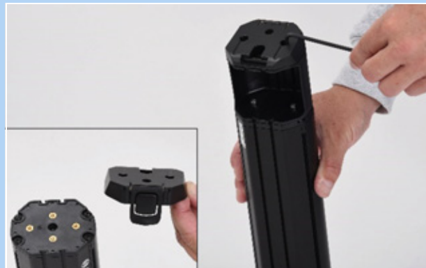
Figure 64: Fastening the battery mounting plate
