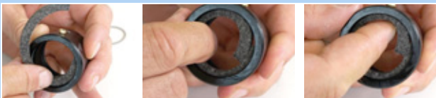
Figure 209: Inserting the felt ring
