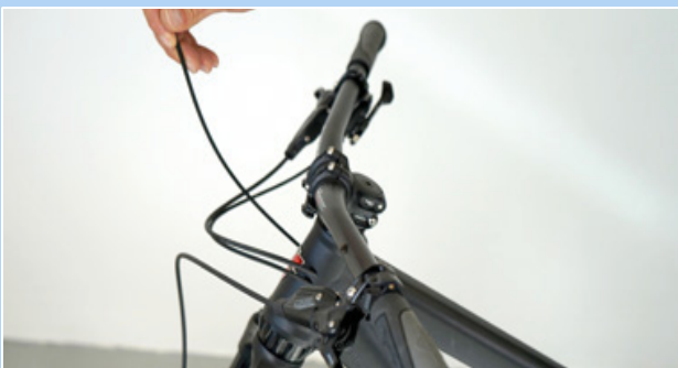
Figure 220: Attaching the end cap
