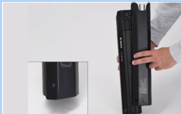
Figure 65: Pushing the battery cover onto battery
