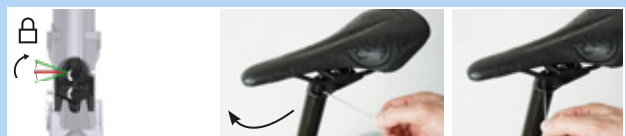
Figure 198: Closing the height adjustment
