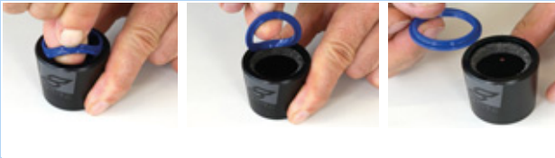
Figure 206: Removing the wiper
