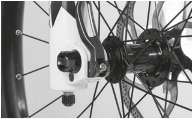
Figure 158: Adjusting the quick release clamping force
